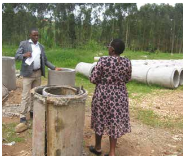
Sheema MC: The municipality was making its own concrete pipe culverts using moulds and trained labourers.
