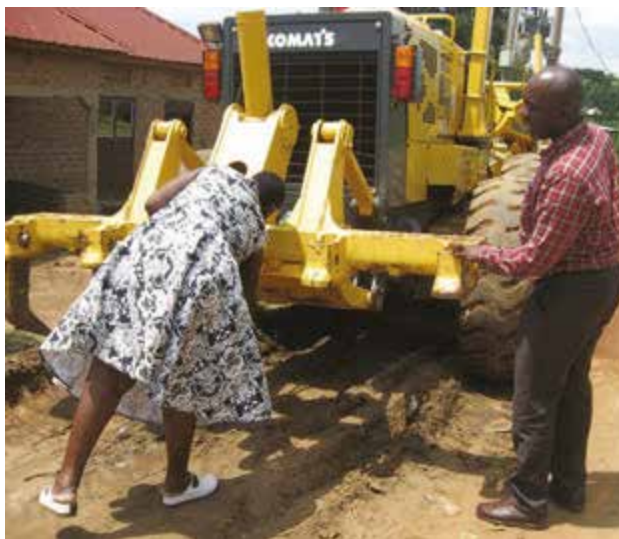
Manafwa district: A motor grader on Bukhaweka-Butiru road (8.8 km) lacking some scarifier teeth due to limited funds.
