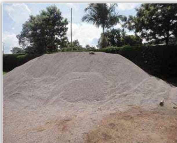
Mukono MC: Sand and stone dust materials procured for the second seal on the 1km section of Nabuti- Nsube road (5km)
